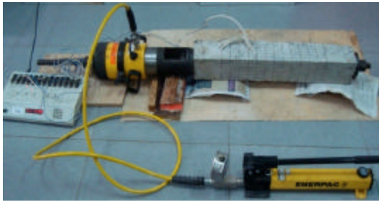
Fig. 2: Applying the sustained load
