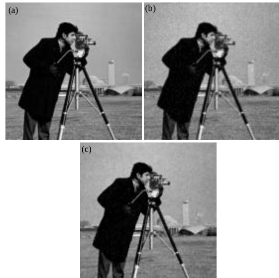
Fig. 2(a-c): Image deblurring for Cameraman. (a) Original image, (b) Degraded image and (c) TV deblurring image
