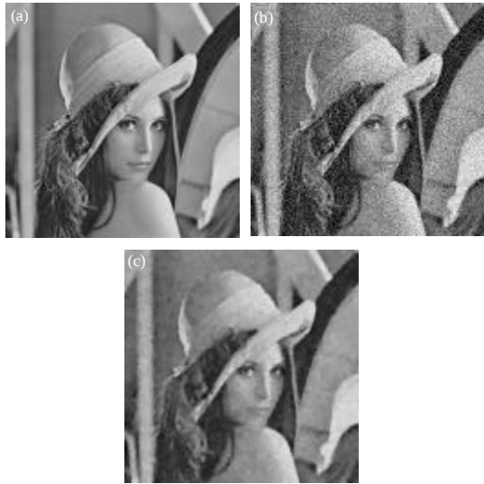
Fig. 4(a-b): Image super-resolution for Lena. (a) Original image, (b) Degraded image, (c) TV super-resolution image
