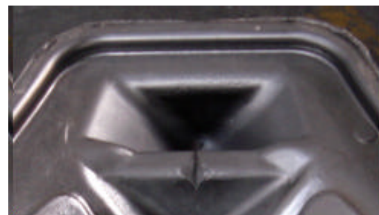
Fig. 5: Folding defect by scheme 1 with experiment
