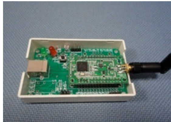
Fig. 4: Real product of the universal WSN node
