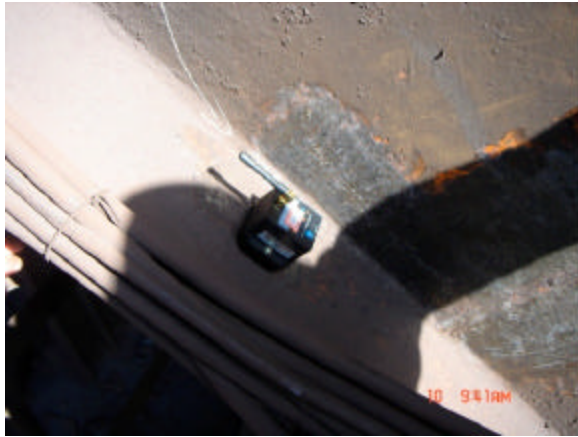
Fig. 10: Arrangement of the acceleration test transducers
