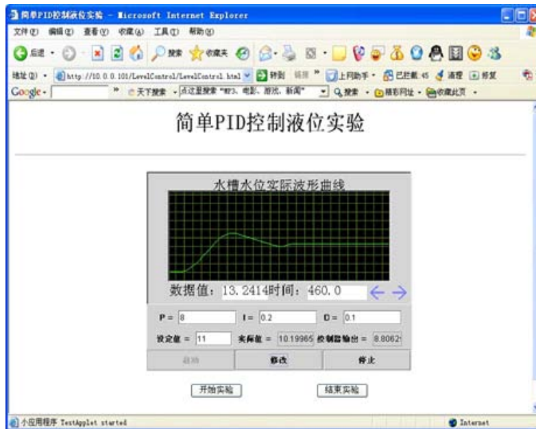
Fig. 13: Remote control results shown on the web client
