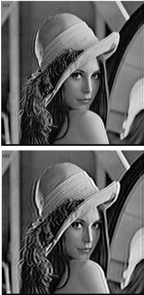
Fig. 6(a-d): Reconstructed SR images at different estimated motion distance. (a) \hat{L} = 1 , PSNR = 34.9869dB, (b) \hat{L} = 2.3501 , PSNR = 39.8186dB, (c) \hat{L} = 3 , PSNR = 34.9968 dB and (d) \hat{L} = 5 , PSNR = 33.5561 dB
