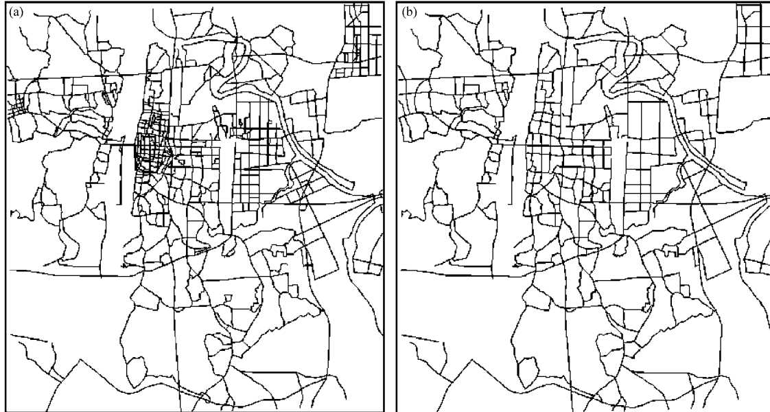
Fig. 5 (a-b): Comparison between data sets at different scales, (a) 1:50, 000 scale data used, (b) Generalization result of 1:100, 000 scale
