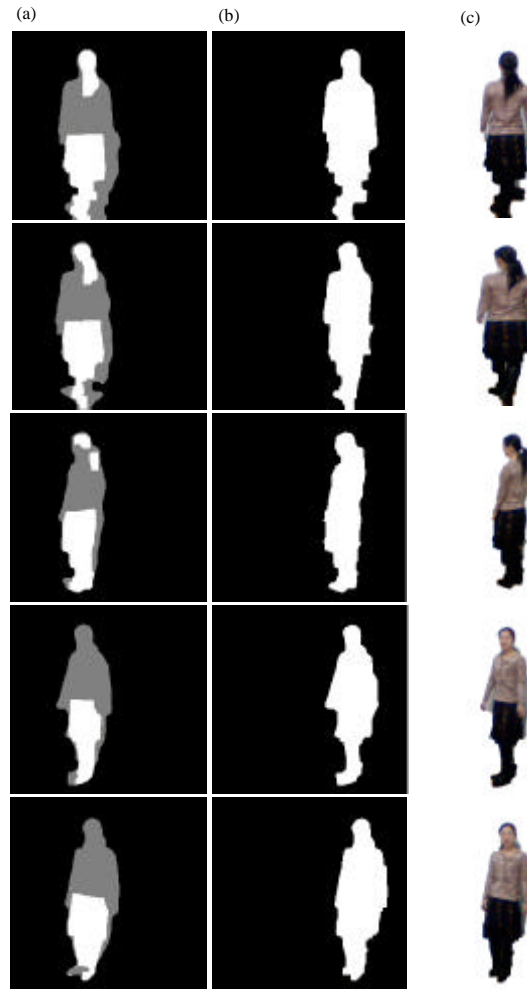
Fig. 4(a-c): Shadow detection compared with normalized rgb, (a) Nnormalized rgb, (b) The proposed method and (c) The extracted objects, respectively. The white regions indicate foreground
