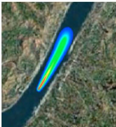
Fig. 8(a-b): Simulation for a sewage outfall in a river, (a) Simulation results within 2 h and (b) COD curve along the river
