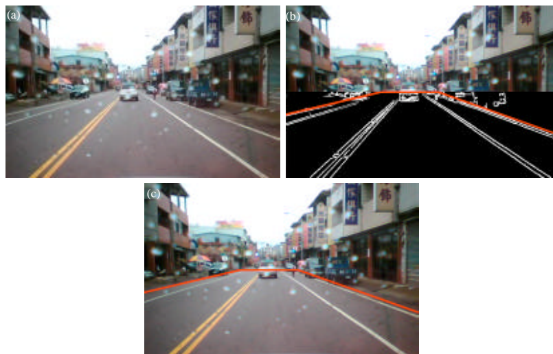
Fig. 4(a-c): Example of traffic lane detection, (a) Original frame, (b) Detection result and (c) The separation of roadway and building areas
