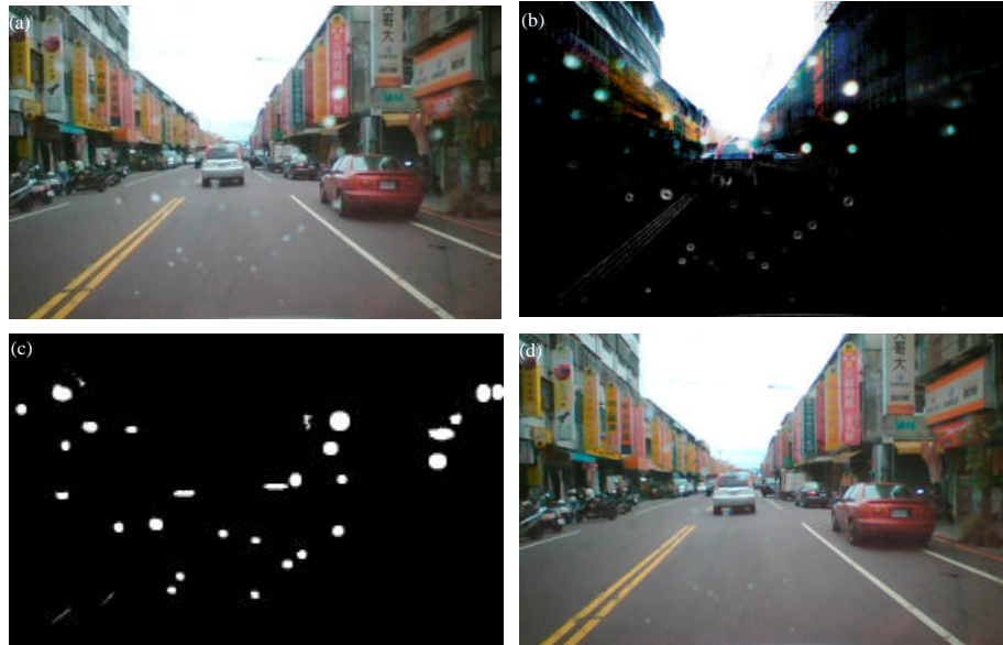
Fig. 13(a-d): Example of removal of a medium number of water drops, (a) Original, (b) Intersection, (c) Detected water drops and (d) Result
