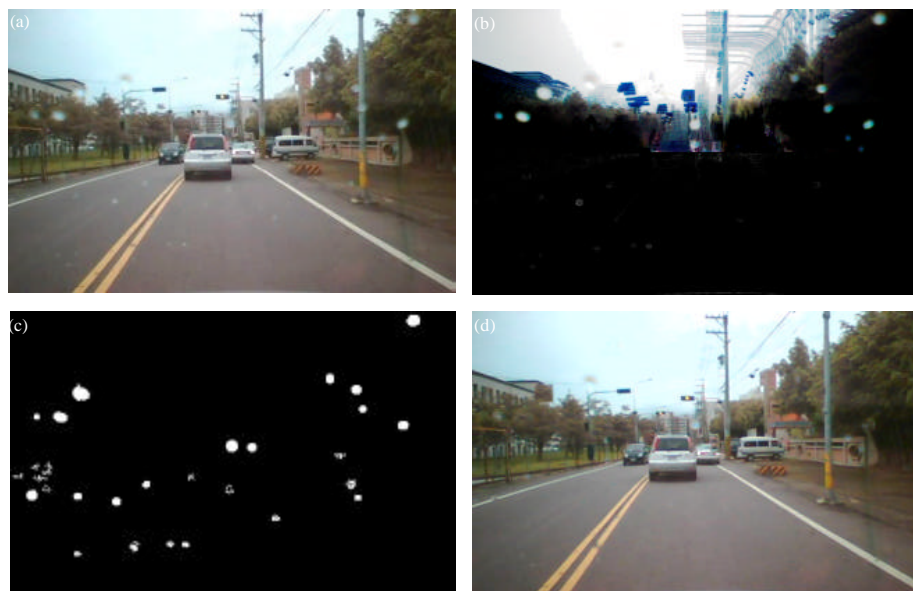
Fig. 12(a-d): Example of removal of a small number of water drops, (a) Original, (b) Intersection, (c) Detected water drops and (d) Result
