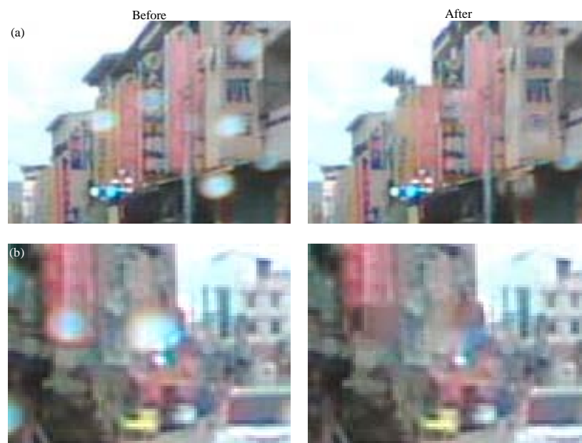
Fig. 11(a-b): Two special cases using image inpainting directly, (a) Template matching failure and (b) Water drops close to the vanishing point
