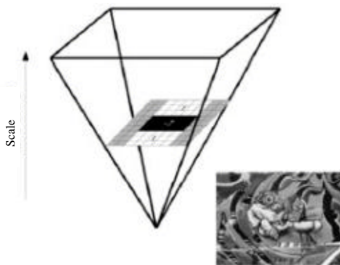
Fig. 2: Image pyramid established by SURF
