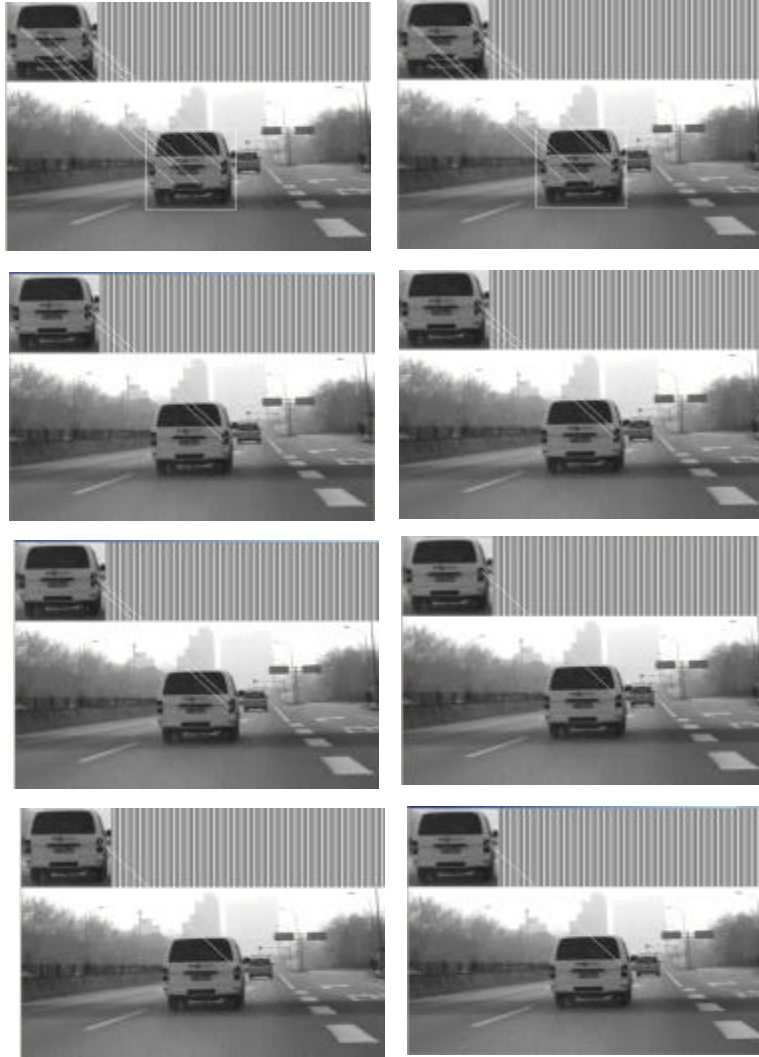
Fig. 5: Feature matching results under different hessian thresholds (hessian thresholds from the first to the last image are: 1500, 2000, 2500, 3000 , 3500, 4000, 4500, 5000 )
