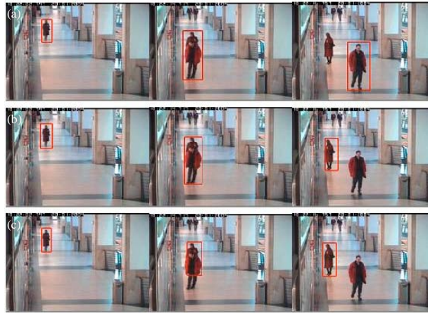
Fig. 1(a-c): Track results of human movement in the similar background environment (a) Single color feature based on PF, (b) Multi-features fusion based on PF and (c) Multi-features fusion based on proposed algorithm
