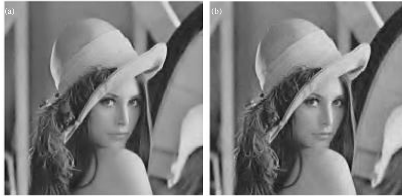
Fig. 10(a-b): (a) Denoised image using the filterbanks in Selesnick and Abdelnour (2004) PSNR = 28.2059 dB and (b) Denoised image using the filterbanks in Table 3 PSNR = 28.4709 dB
