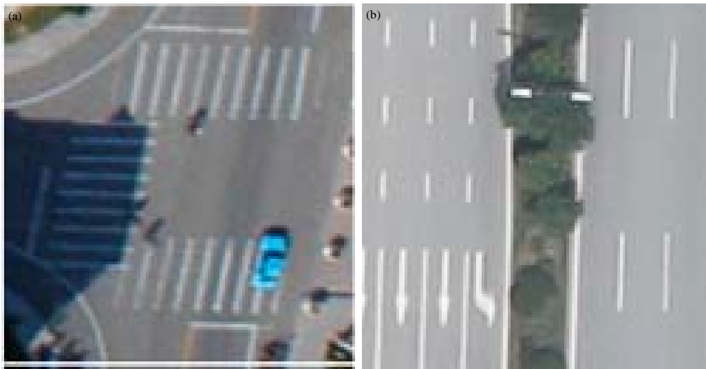
Fig. 6(a-b): Subsection of an image with motion blur (left) and the de-blurred image result (right) of an image with controlled stabilized platform and shorter exposing time
