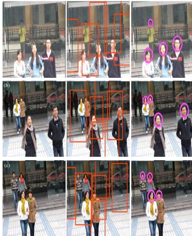
Fig. 2(a-c): Contrast of detection results (a)Original image (b)HOG detection and (c)MB-LBP detection
