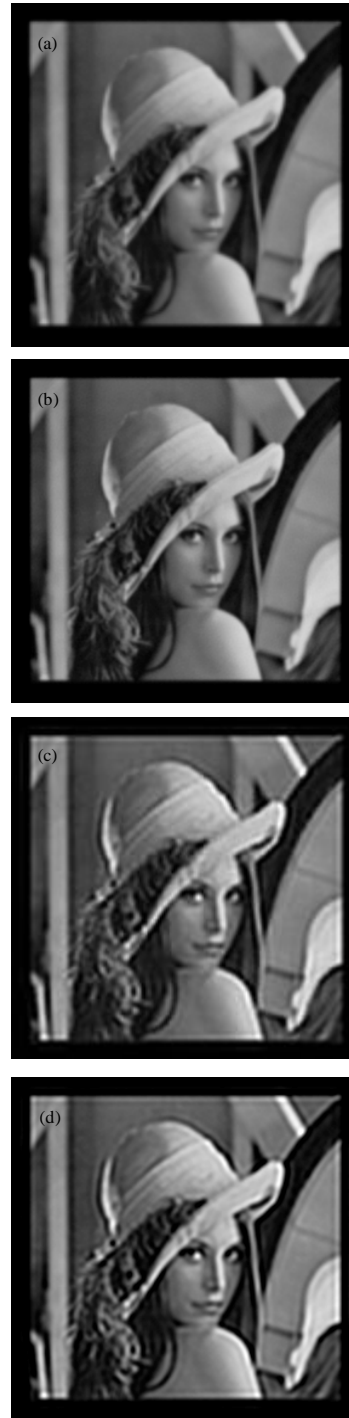
Fig. 6(a-d): The reconstructed images through bilinear interpolation and super-resolution at different standard deviations ( \hat{\kappa} = 7 ), (a) Bilinear interpolation (PSNR = 33.7897 dB), (b) SR image ( \hat{\sigma} = 0.1 , PSNR = 34.6452 dB), (c) SR image ( \hat{\sigma} = 1.19 , PSNR = 35.4701 dB) and (d) SR image ( \hat{\sigma} = 4 , PSNR=33.0961 dB)
