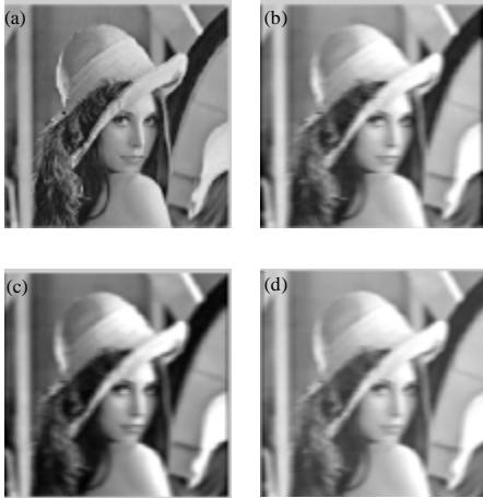
Fig. 2(a-d): Restored results for (a) Original (b) Degraded (c) Restored by MNNs and (d) Restored by median filter fuzzy image
