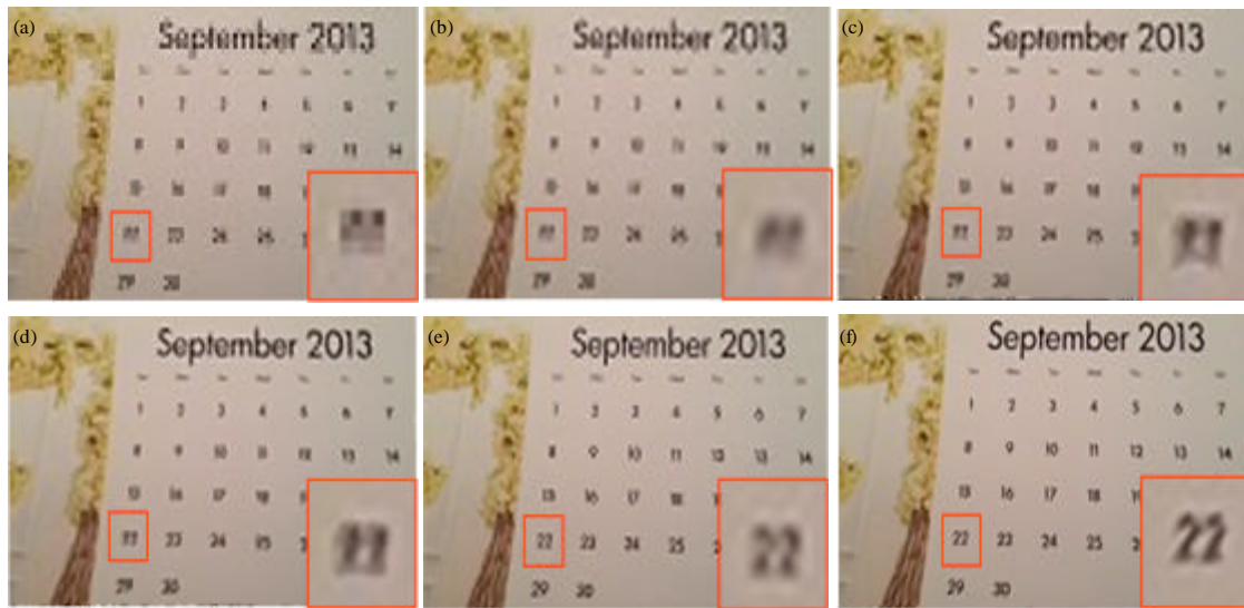
Fig. 3(a-f): Example estimated HR estimation from different super resolution methods. Results (3x resolution increase) by (a) Original low resolution image interpolated by nearest neighbor interpolation, (b) Bicubic interpolation, (c) Fast and robust method, (d) TV reconstruction, (e) Normalized convolution and (f) Proposed method
