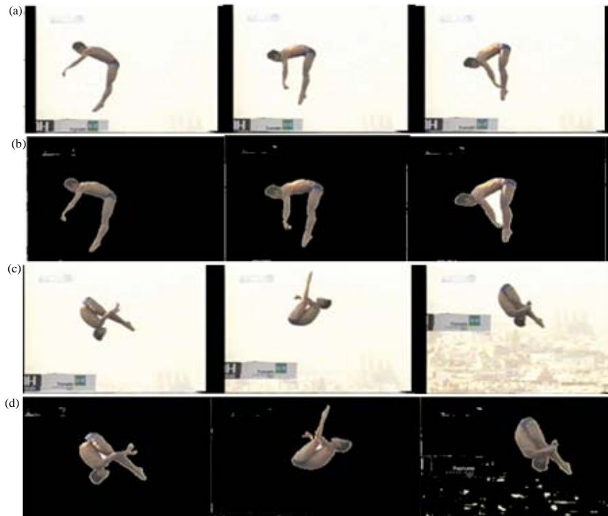
Fig. 10(a-d): Diving video segmentation results (a, c) Original video sequence and (b, d) Segmentation results
