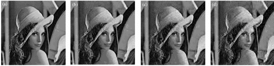
Fig. 5(a-d): For different compression ratio, the reconstruction effects of signal when the reconstructed algorithm run in cloud, (a) Original image, (b) Reconstructed image (N:M = 2:1), (c) Reconstructed image (N:M = 3:1) and (d) Reconstructed image (N:M = 4:1)
