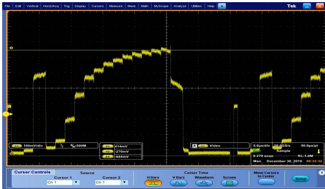
Fig. 4: Grayscale waveform diagram when the amount of light of A camera increases of 3.5 files
