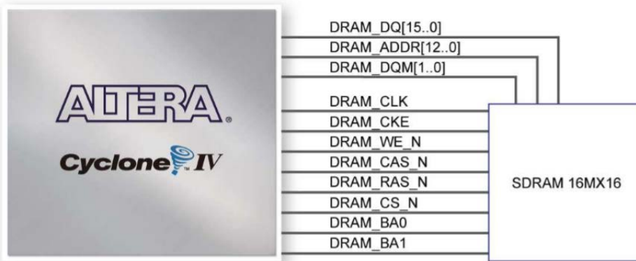
Fig. 4: Connections between FPGA and SDRAM
