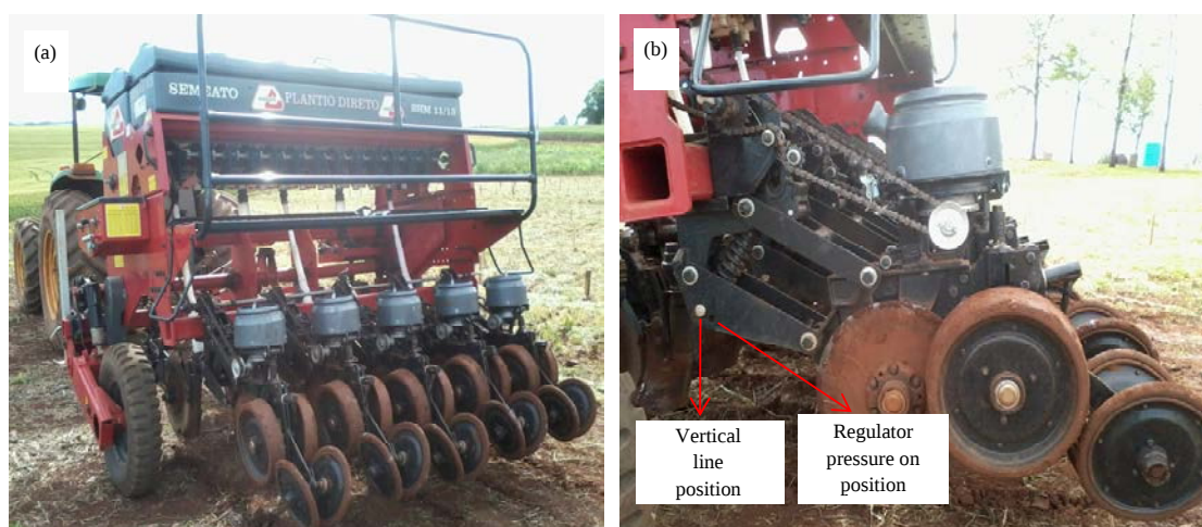
Fig. 1(a-b): Seed-drill used at the experiment, as follows, (a) Seed-drill semeato brand, model SHM and (b) Pantograph system of lines with their respective regulator pressure on vertical line position
