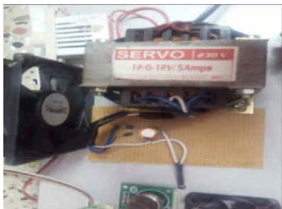
Fig. 7: Transformer (12v-5 A range) with cooling fan
