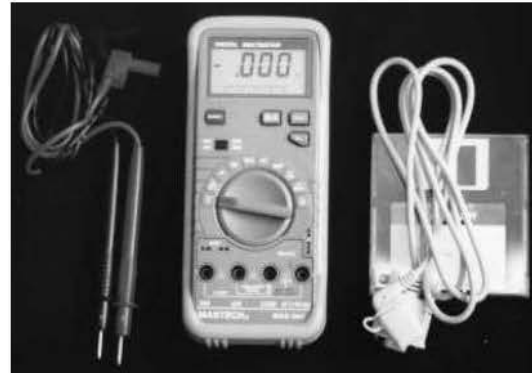
Fig. 7: Multi-meter used for measuring the electric voltage and the electric current
