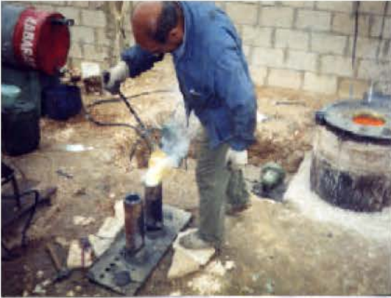
Fig. 1: The blast furnace of melting copper and the traditional way to pour down the mass inside the mold
