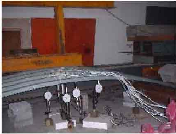
Fig. 4: Setting of deformation gauge, LVDT and strain gauge
