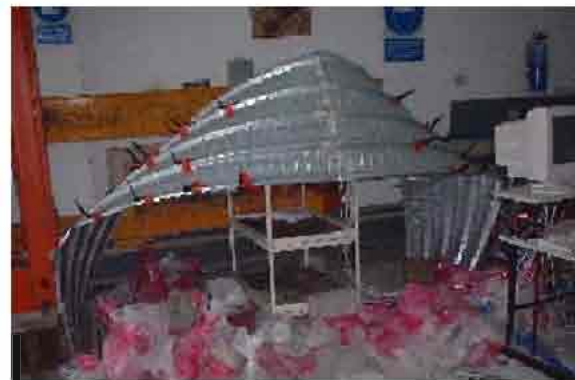
Fig. 14: Experimental deflected shape of cylindrical roofing element
