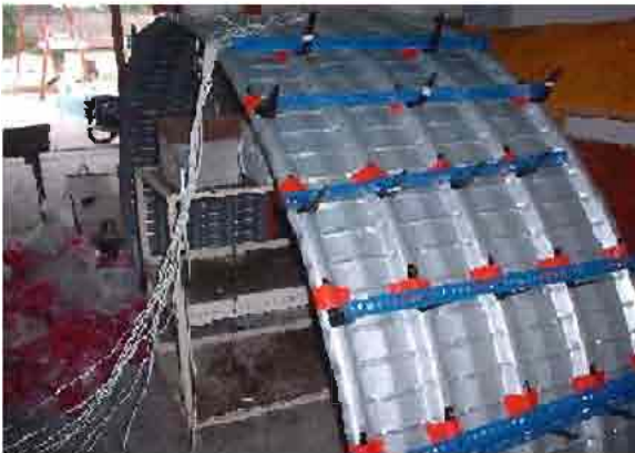
Fig. 5: Test setup for cylindrical shell roofing elements
