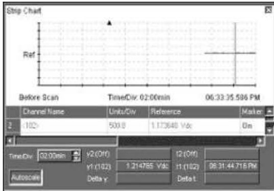
Fig. 3: Snapshot of data logger software showing radiometer output voltage for clear sky (1.214 v)
