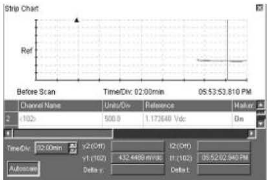
Fig. 5: Snapshot of data logger software showing radiometer output voltage for rainy clouds (0.432 v)
