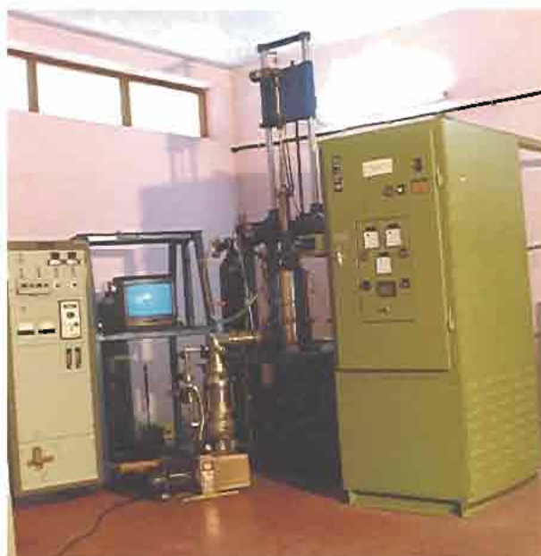
Fig. 1: Czochralski crystal growth workstation
