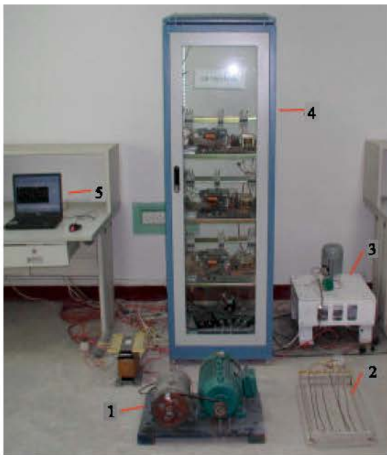
Fig. 8: Experimental system. (In the picture: 1-wind generation simulator unit including an induction motor and a permanent magnet synchronous generator; 2-DC load; 3-flywheel energy storage unit; 4-converters and control system; 5-control computer)
