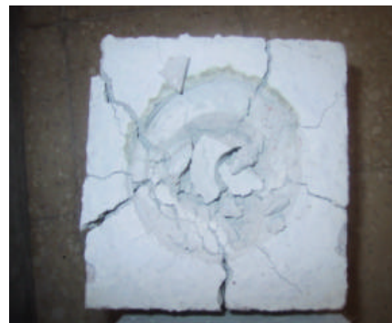
(b) Pullout test sample after burning
