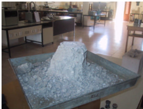
(b) The concrete cube after one day from the testing time Fig. 6a and b: Concrete behavior at temperature of 1000°C, before and after collapsing
