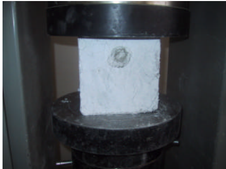
(a) The concrete cube exactly the moment of testing
