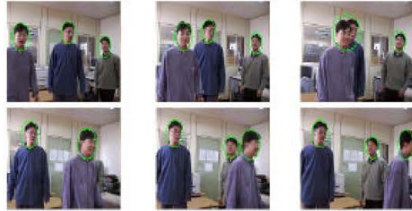
Fig. 5: Tracking in case of closing two faces
