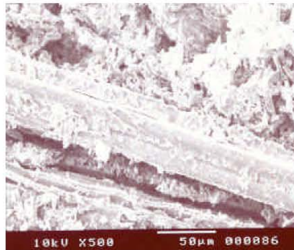
Fig. 2a: Electromicroscope analysis of composite material obtained in serial 2
