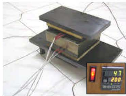
Fig. 2: Photograph of the compression-molding machine with the control system
