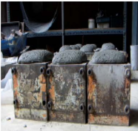
Fig. 2: Mould filled with AC mix upto 80% of depth (ppox.)
