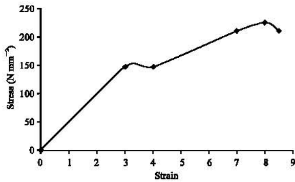
Fig. 3: Stress-strain curve for HTMT 97.99% deformation
