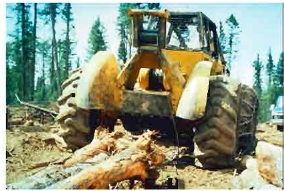
Fig. 4: A rubber-tired chained skidder in skidding operation
