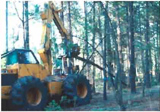
Fig. 3: Delimiting and bucking the trees with double-grip harvester
