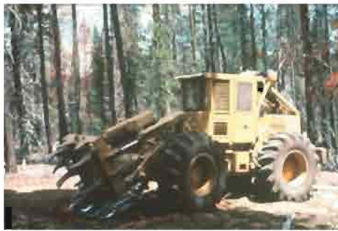
Fig. 2: A rubber-tired feller-buncher in felling operation
