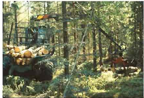
Fig. 6: Forwarders equipped with a hydraulic grapple loading arm
