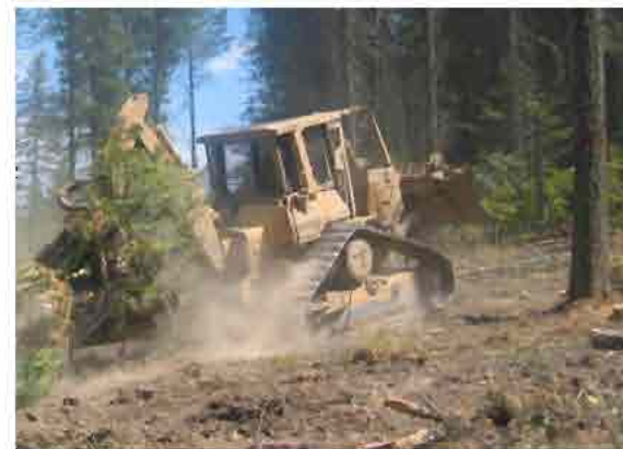
Fig. 5: Ground skidding with a crawler tractor using grapple
