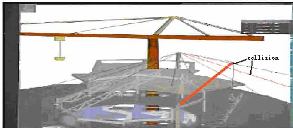
Fig. 2: Collision occurred between the secondary mast and the cable
