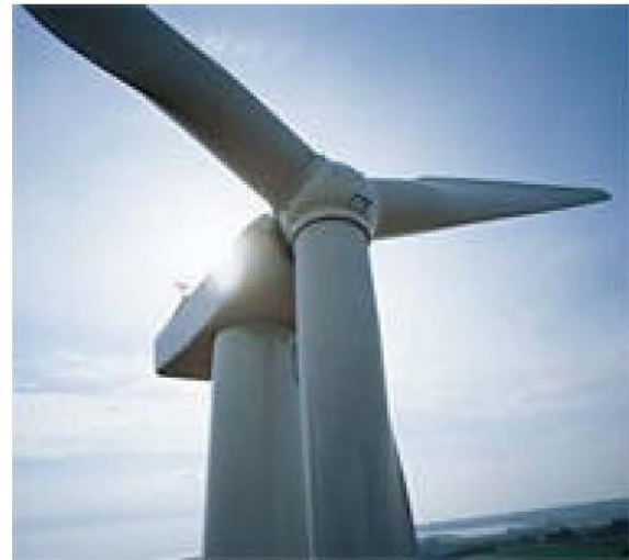
Fig. 3: A blade that is upright and away from the shadowing effects of the tower is exposed to quite different loads from a blade that is pointing downwards
