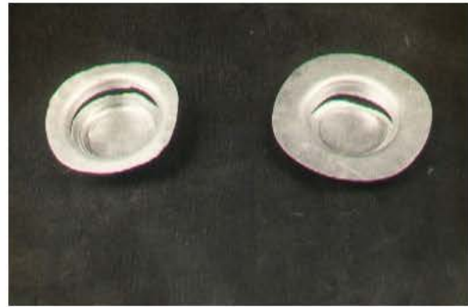
Fig. 5: Broken cup due to low ductility of materials on the left is material deformed 80%, Annealed at 300 °C for 2 1/2 h. 60/33 die used on the right is material deformed 90%, annealed at 400 °C for 2 h. 65/33 deep drawing die used
