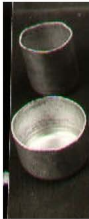
Fig. 3: One set of cups showing no earing at the rims. The set was deep drawn from 90% cold-rolled Aluminium 1200 sheet annealed at 460 °C for 4 h, respectively
