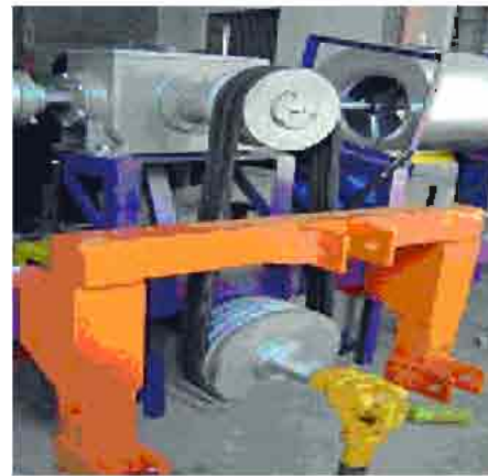
Fig. 2: Power train system from tractor PTO to the fans
