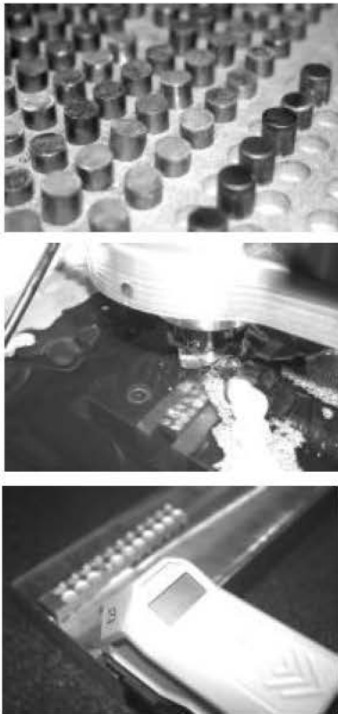
Fig. 3: Copper electrodes ( \phi 10 \times 10 mm) and surface roughness measurement device
