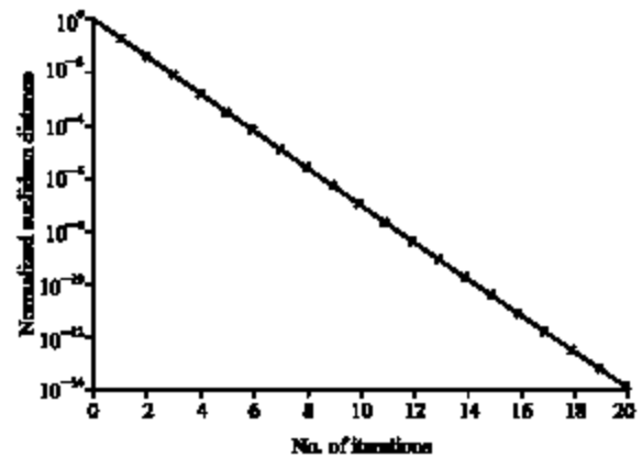
Fig. 4 Convergence of Distributed Power Control (DPC), SIR = 1 dB
