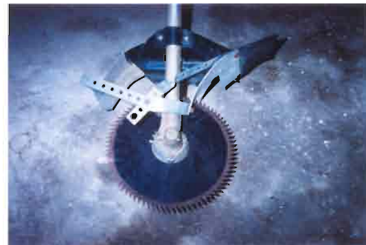
Fig. 2: Blade assembly of the rice harvester
