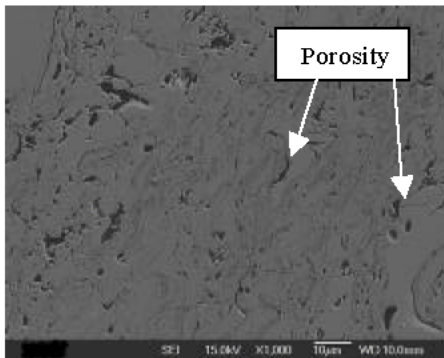
Fig. 1: Morphology of FeNb coatings
