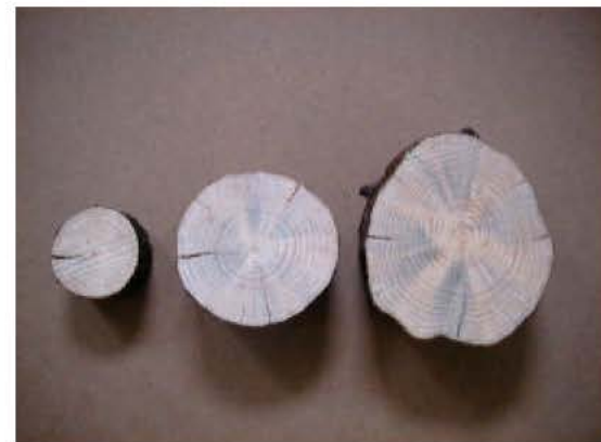
Fig. 2: Blue stain defects were encountered on sample timber segments obtained from a fire-killed Brutian pine tree
