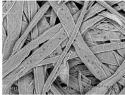
Fig. 2: SEM image of sheet made from the pulp having (14 °SR)
