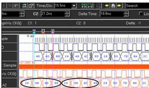
Fig. 7: 90 MHz output waveform of the logic analyzer
