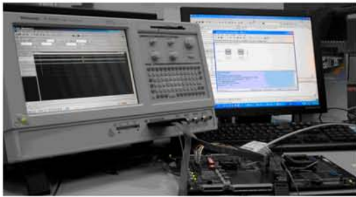
Fig. 6: FPGA implementation and verification platform
