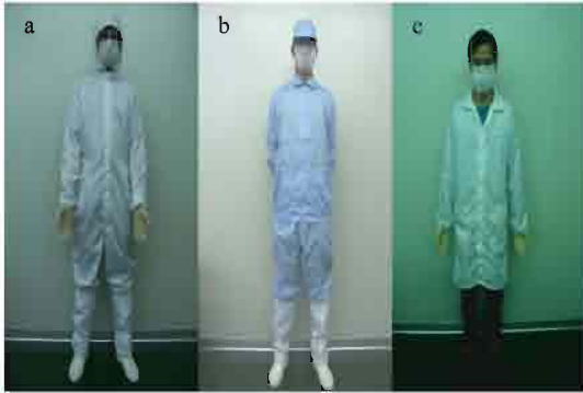
Fig. 4: Types of garment system for testing (a) attached hood coverage (b) two piece suit and (c) cleanroom coat
